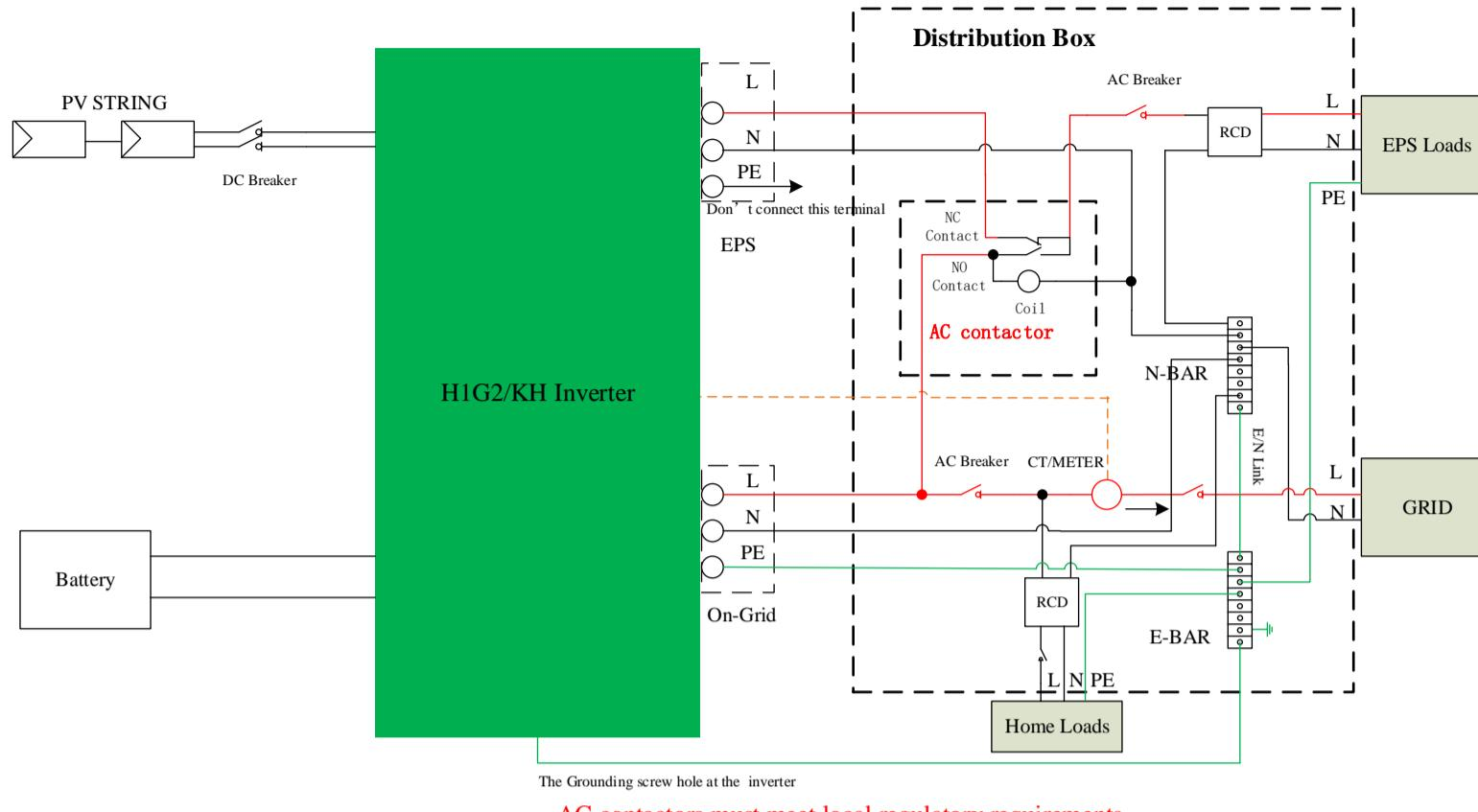
Neutral line of alternative supply must not be isolated or switched.
